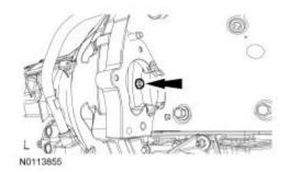
6. Install the starter motor dust shield and install the 2 retainers.
