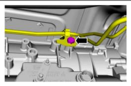
Remove the wiring harness retainer from the transmission and position the wiring harness aside.
