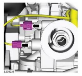
5. Remove the wiring harness bracket nut and position the wiring harness aside.
