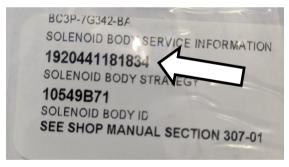
43. If the decal is missing. Remove the transmission pan and copy the note from the tag installed onto the valve body.
