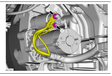
11. Remove the nut and position the wiring harness aside.
