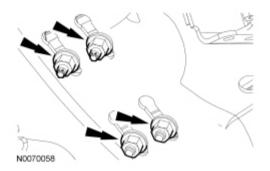
21. Remove the 3 LH engine support insulator nuts.
