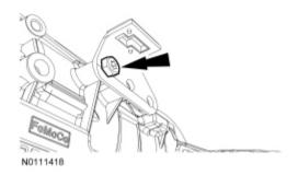
27. Disconnect the 3-position mode switch electrical connector.
