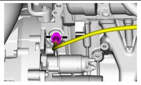
33. Secure the wiring harness and tighten to 12 Nm (106 in-lb).
