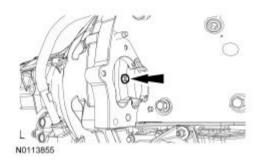
16. Rotate the shell of transmission vehicle harness connector counterclockwise and disconnect the transmission vehicle harness connector.
