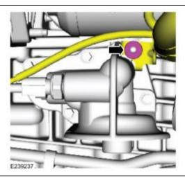
6. Remove the stud bolt, the bolts and the oil filter adapter.
