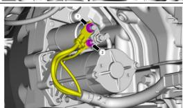
36. Install the starter motor cable cap.
